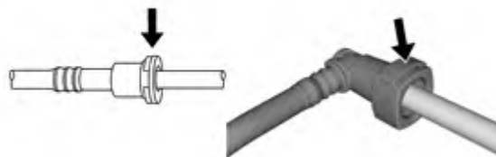
Fig. 66: Variants Of Sliding Retainer Style Connectors Courtesy of GENERAL MOTORS COMPANY
